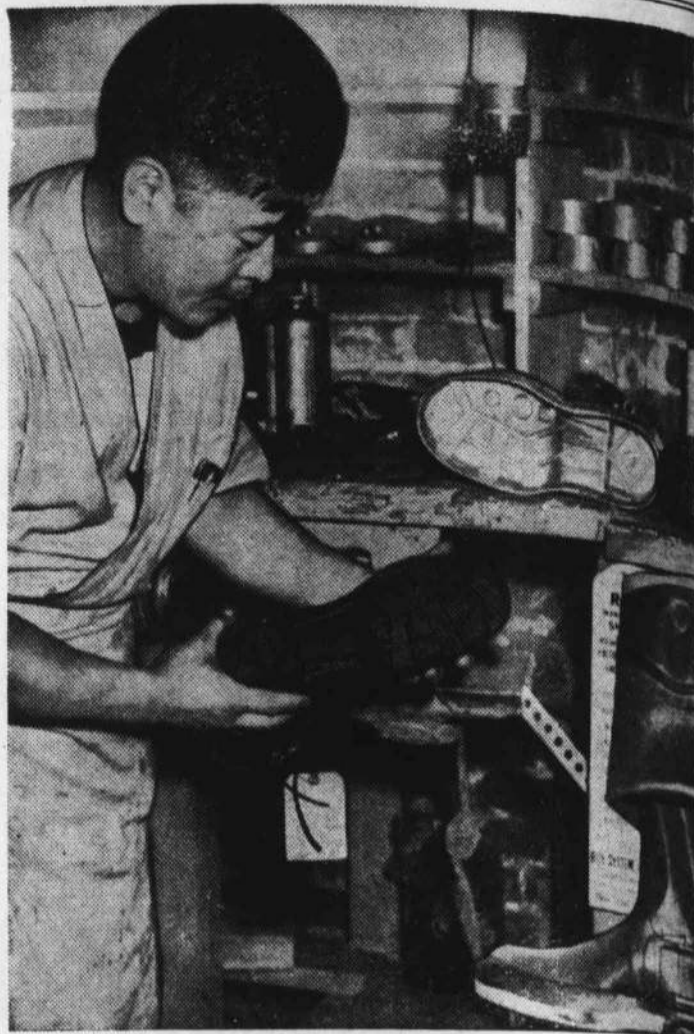
Joe Suyama of Denver demonstrates three types of boot resoling he has perfected. He is holding an industrial sole, the mold for which lies on the bench. Near the mold is a raw cord sole. At right is a felt-resoled boot which fishermen have hailed enthusiastically. So far as Suyama knows, his is the first shoe repair shop to resole ordinary rubber fishing boots with felt. Suyama designed his own molds and cast them out of aluminum. He also designed his own press which develops a ton and a half pressure, and wired it to provide the 280-degree temperature required. Suyama declares he has resoled with felt several thousand pairs of boot waders in the last three years without complaint because of his vulcanizing process. Fishermen like the felt soles to keep from slipping while wading in algae covered stream beds. —Cut courtesy Denver Post
